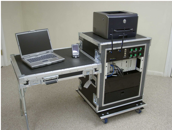
Vehicle Data Acquisition Test System Figure 2
